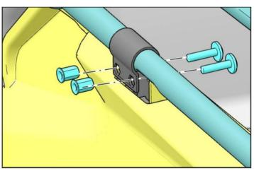
5. After installing the door panels and reattaching the door liners with fasteners for fastening.
