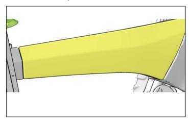
3. Place the left ( right ) door cutting tool on the door liner at a suitable position ( the position shown in the figure below), draw the outline of the tooling on the liner and cut the liner here with the tool.
