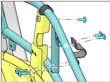
4. Secure the front of the half-door ASSY with the lower half-door adapter bracket , using the bolt and flat head hexagonal rivet nuts to the door bracket.
