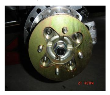
\*2. Put the hub spacer on the ATV hub.
