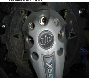
6. Position the sprocket of the XGEN assembly to allow the sprocket to fully engage into the hub adaptor.
